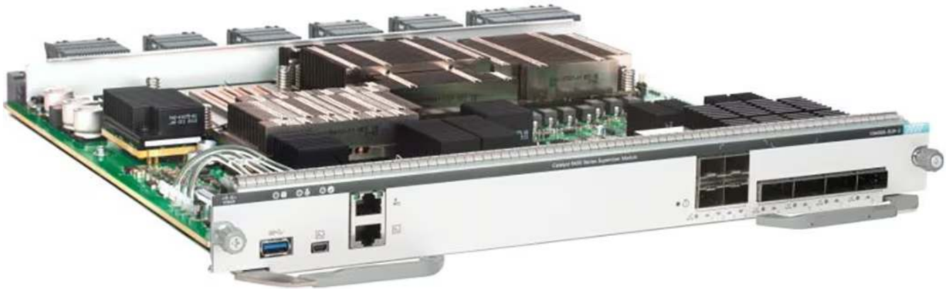
Figure 2. C9400X-SUP-2 supervisor engine
